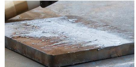
After the attachment is removed, operators can reduce the amperage on the system and wash any remaining material away without digging into the workpiece. FlushCut washing further reduces the need for grinding.
