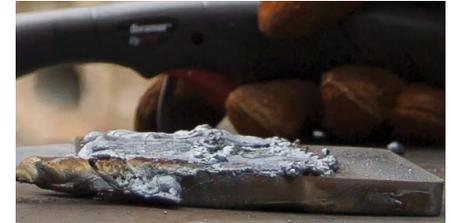
When using FlushCut consumables, operators can expect to leave less than 5 mm (3/16") of material on the workpiece after the removal of a lug, attachment or pad eye.
